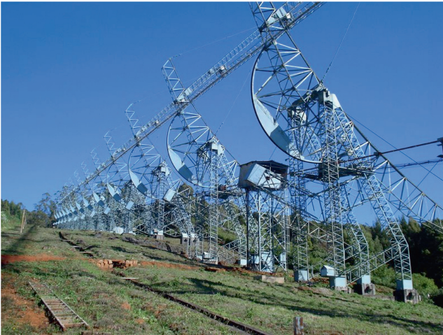
Figure 1. The Ooty Radio Telescope is an offset cylindrical paraboloid, 530 m \times 30 m in size. It is equatorially mounted. The Ooty Wide Field Array (OWFA) is an upgrade to the ORT, which digitizes the signals from every 4 dipoles along the feed line. These signals are then cross-correlated, leading to a very wide field-of-view interferometer. See text for more details.
